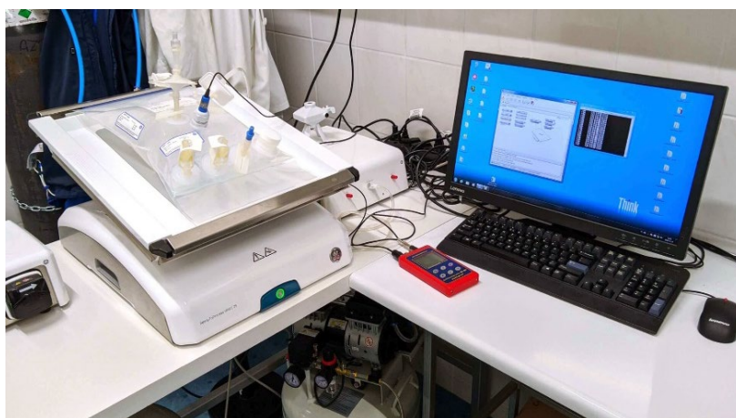
Fig. 1. Experimental setup: ReadyToProcess WAVE 25 bioreactor and the CX-401 meter connected to a computer.
