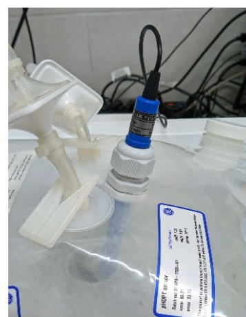
Fig. 2. pH electrode mounted on the Cellbag 2 L vessel.
