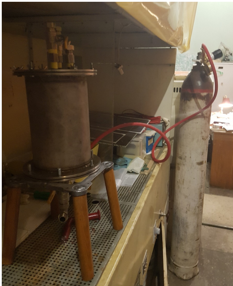
Fig.1. The pilot-laboratory installation for research the process of catalytic hydration of acetylene.
