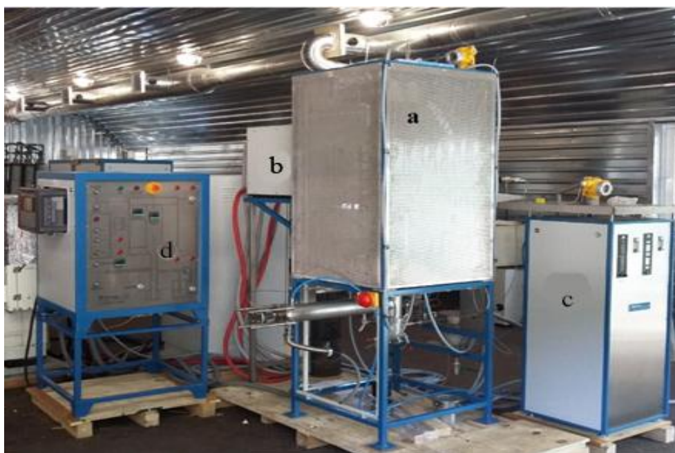
Fig. 2. Experimental pyrolysis installation manufactured by the German company Linn High Them [8].
